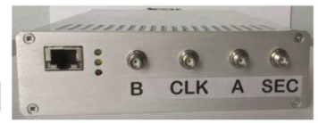
Fig. 9. Front view of the ADR box, that contains the boards displayed in Fig. 8. The input labels correspond to those of Fig. 6 (with for A = input 1 and B = input 2). The receiver can operate independently in a section of the radio telescope or installed in the ADR Server).
