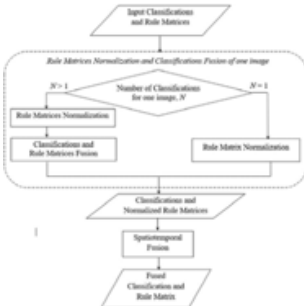
Figure 1. Dataflow diagram of spatiotemporal fusion of land cover classifications based on probability propagation inference that represented as rule matrices
