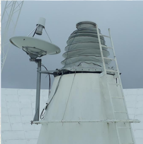
Feed antenna at secondary focus of RT-32 – tripple mirror system
